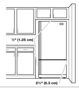
To ensure proper ventilation for your refrigerator, allow for a  $\frac{1}{2}$ " (1.25 cm) space on each side and at the top. Allow at least 1" (2.54 cm) between back of cabinet and the wall. If your refrigerator has an ice maker, allow extra space at the back for the water line connections.
