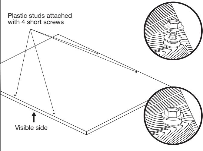
Attach the 4 plastic studs to the wooden panel using the four  $\frac{5}{16}$ " hex-head (short) screws provided.
