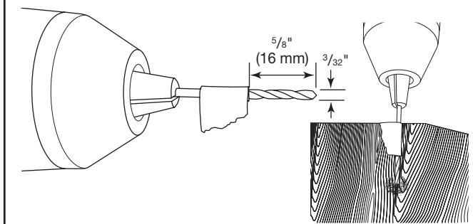
**NOTE:** Do not drill deeper than  $\frac{5}{8}$ " (16 mm) to keep from drilling through panel. Pilot hole depths given are for  $\frac{3}{4}$ " (19 mm) thick panel.
