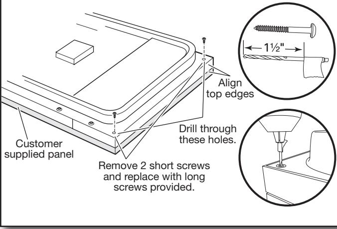
Open the door and align top edges. Use tape to mark a  $\frac{3}{32}$ " drill bit to gauge the hole depth of approximately  $1\frac{1}{2}$ " (38 mm). Drill pilot holes into the top corners of the door, using hole in liner as a guide.
