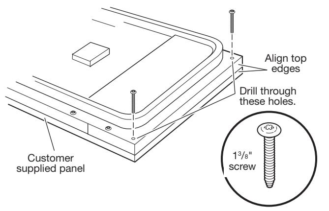
Using a Torx® T15® screwdriver, install two #8 x 1<sup>3</sup>/<sub>8</sub>" (long) screws in top corners to secure custom wood panel in place.
