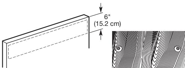
Install the custom hardware handle(s) on the front of the wooden panel inside dotted line.
