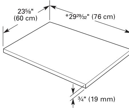
\*This dimension is for 4" (102 mm) toekick. If the installation needs a higher toekick, adjust the height of the wood panel accordingly except on models with fan-assisted dry. Fan models may have a duct at the bottom of the door that would be exposed if you shorten the door panel for toekick heights above 4" (102 mm). Toekick heights greater than 6" (152 mm) are not recommended for this product.
