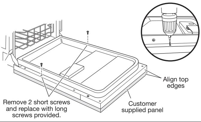
Remove the short screws (3rd from top) on either side of the inner door panel. Use tape to mark a  $\frac{3}{32}$ " drill bit to gauge the hole depth of approximately 1 $\frac{1}{2}$ " (38 mm). Drill 2 pilot holes using the door liner hole as a guide into the panel. Install the 2 remaining long screws.
