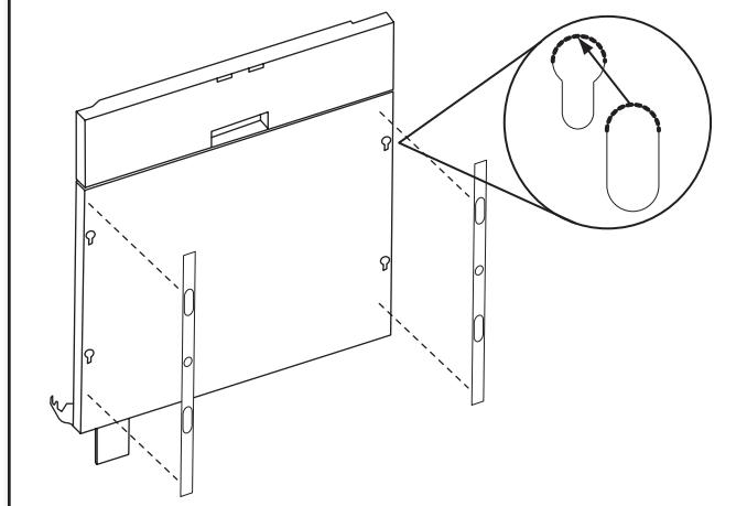
Check custom tape alignment with metal door slots; verify tape is right-side up and that the tape does not overhang the metal door on the top, bottom, or side interfaces. Remove the backing from the custom tape by pulling straight down on the liner. Align the custom tape to the keyhole slots on the metal door (see the previous illustration) and apply. Repeat steps for one side and then the other.
