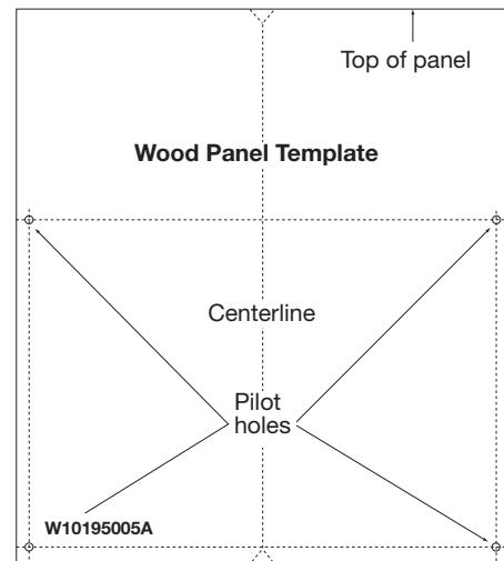
Using the template provided, attach it to the backside of the custom panel with tape. Make sure that the center of the template is aligned with the center of the wooden panel and top of the template is aligned to the top face of the wooden panel.
