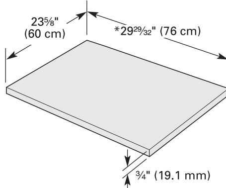
\* This dimension is for 4" (10.2 cm) toe kick. If the installation needs a higher toe kick, adjust the height of the wood panel accordingly except on models with fan assisted dry. Fan models have a duct at the bottom of the door that would be exposed if you shorten the door panel for toe kick heights above 4" (10.2 cm). Toe kick heights greater than 6" (15.2 cm) are not recommended for this product.
