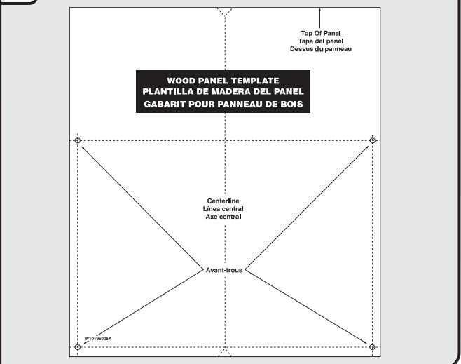
Using the template provided, attach it to the backside of the custom panel with tape. Make sure that the center of the template is aligned with the center of the wooden panel and top of the template is aligned to the top face of the wooden panel.
