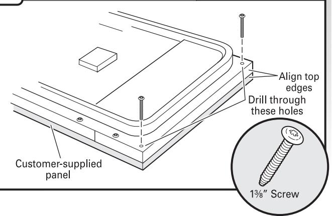
Using a Torx® T15® screwdriver, install two #8 x  $1\frac{1}{8}$ " screws in top corners to secure custom wood panel in place.
