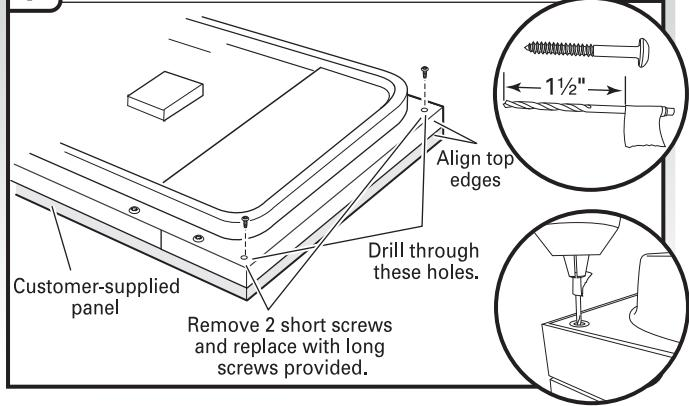
Open the door and align top edges. Use tape to mark a  $\frac{3}{32}$ " drill bit to gauge the hole depth of approximately  $1\frac{1}{2}$ " (3.8 cm). Drill pilot holes into the top corners of the door, using hole in liner as a guide.
