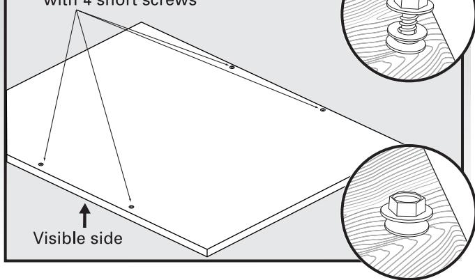
Attach the 4 plastic studs to the wooden panel using the four  $\frac{5}{16}$ " hex-head (short) screws provided.
