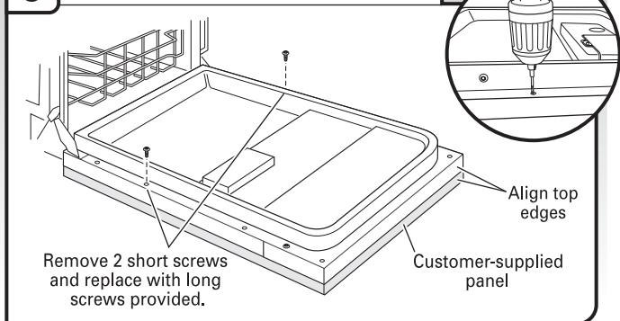
Remove the short screws (3rd from top) on either side of the inner door panel. Use tape to mark a  $\frac{3}{32}$ " drill bit to gauge the hole depth of approximately  $1\frac{1}{2}$ " (3.8 cm). Drill 2 pilot holes using the door liner hole as a guide into the panel. Install the 2 remaining long screws.
