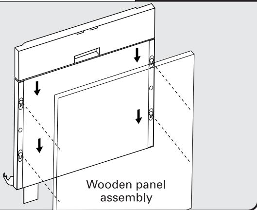
Align the studs on the custom wood panel to the keyhole slots on the door assembly. Ensure that all 4 plastic studs are engaged in the keyhole slots. Slide wood panel down until the top surface of the wooden panel is flush with the top of the door.
