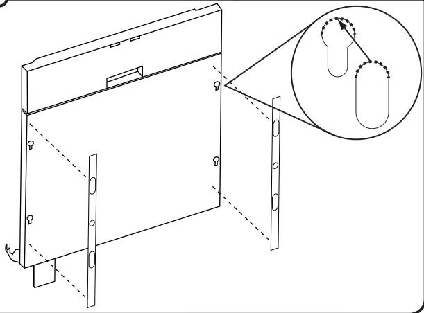
Check custom tape alignment with metal door slots; verify tape is right-side up, and that the tape does not overhang the metal door on the top, bottom or side interfaces. Remove the backing from the custom tape by pulling straight down on the liner. Align the custom tape to the keyhole slots on the metal door (see the previous illustration) and apply. Repeat steps for one side and then the other.
