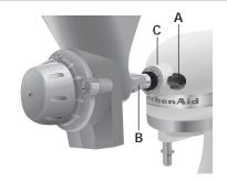
2. Insert the attachment shaft housing (B) into the attachment hub (C), making certain that the power shaft fits into the square hub socket. Rotate the attachment back and forth if necessary. When the attachment is in proper position, the
