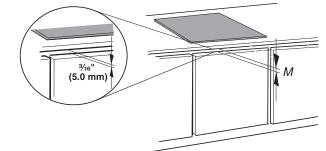
**NOTES:** After you make the countertop cutout, some installations may require notching down the base cabinet side walls to clear the cooktop base. To avoid this modification, use a base cabinet with sidewalls wider than the cutout.
