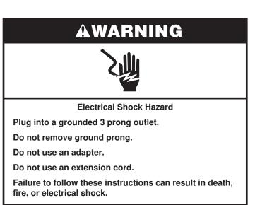
**Electrical:** A 115 V, 60 Hz., AC only, 15 or 20 A fused, grounded electrical supply is required. It is recommended that a separate circuit serving only your freezer be provided. Use an outlet that cannot be turned off by a switch. Do not use an extension cord.
