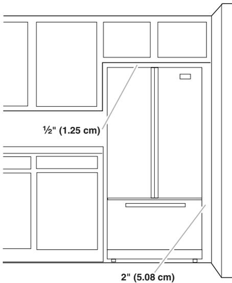
To ensure proper ventilation for your refrigerator, allow for a 1/2" (1.25 cm) of space on each side and at the top. Allow for a 1" (2.54 cm) space behind the refrigerator. If your refrigerator has an ice maker, allow extra space at the back for the water line connections. When installing your refrigerator next to a fixed wall, leave a 2" (5.08 cm) minimum space between the refrigerator and wall to allow the door to swing open.
