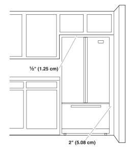
To ensure proper ventilation for your refrigerator, allow for a 1/2" (1.25 cm) of space on each side and at the top. Allow for a 1" (2.54 cm) space behind the refrigerator. If your refrigerator has an ice maker, allow extra space at the back for the water line connections. When installing your refrigerator next to a fixed wall, leave a 2" (5.08 cm) minimum space between the refrigerator and wall to allow the door to swing open.
