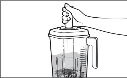
**5** Use the Flex Edge tamper accessory as needed for optimal blending performance. Remove the ingredient-measuring cap only, and leave the lid in place. Stir or press contents down towards the blade. When you are finished, replace the ingredient-measuring cap in the blender jar lid before resuming blending.
