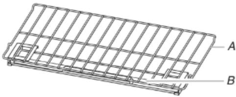
A. Steam rack B. Water reservoir
