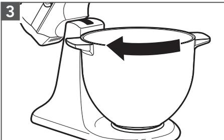
Place the Bread Bowl on the clamping plate to secure in place.
