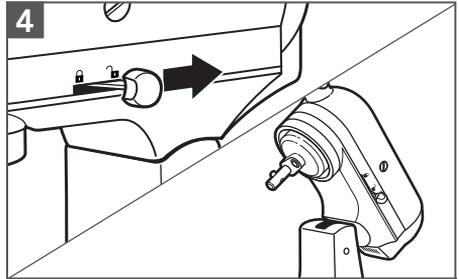
**Raise the Motor Head:** Unlock and lift the Motor Head. Then, lock\* the head to keep it lifted.
