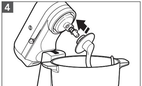
Attach the Dough Hook for your recipe, using the directions in the Stand Mixer Instructions manual. Then place the motor head back in the down position and lock into place.
