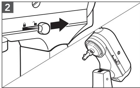
**Raise the Motor Head:** Unlock and lift the Motor Head. Then, lock\* the head to keep it lifted.
