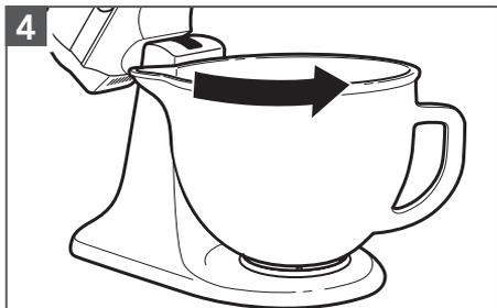
**Remove the Ceramic Bowl:** Twist to unlock the bowl from the clamping plate.
