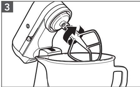
**Remove the accessory:** Press the accessory upward, turn it and pull it away from the beater shaft.
