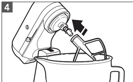
Attach the appropriate accessory for your recipe, using the directions in the Stand Mixer Instructions manual. Then place the motor head back in the down position and lock into place.
