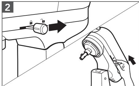
Unlock and lift the Motor Head. Then, lock\* the head to keep it lifted.
