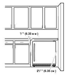
To ensure proper ventilation for your wine cellar, allow for a  $^{1/}$ " (6.35 mm) space on each side and at the top. When installing your wine cellar next to a fixed wall, leave  $2^{1/}$ " (6.35 cm) minimum clearance on the hinge side to allow for the door to swing open.
