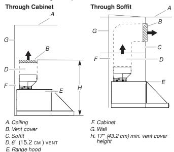
**NOTE:** 12" (30.5 cm) high cabinets without a soffit may allow the 6" (15.2 cm) vent and vent cover to be seen.
