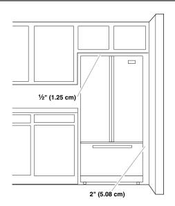
To ensure proper ventilation for your refrigerator, allow for a  $\frac{1}{2}$ " (1.25 cm) of space on each side and at the top. Allow for a 1" (2.54 cm) space behind the refrigerator. If your refrigerator has an ice maker, allow extra space at the back for the water line connections. When installing your refrigerator next to a fixed wall, leave a 2" (5.08 cm) minimum space between the refrigerator and wall to allow the door to swing open.
