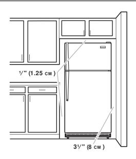
To ensure proper ventilation for your refrigerator, allow for 1/2" (1.25 cm) space on each side and at the top. Allow at least 2" (5.08 cm) between back of cabinet and the wall. If your refrigerator has an ice maker, make sure you leave some extra space at the back for the water line connections.
