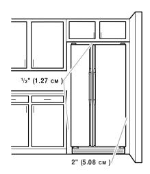
To ensure proper ventilation for your refrigerator, allow for  $\frac{1}{2}$ " (1.27 cm) of space on each side and at the top. Allow for 1" (2.54 cm) of space behind the refrigerator. If your refrigerator has an ice maker, allow extra space at the back for the water line connections. When installing your refrigerator next to a fixed wall, leave a 2" (5.08 cm) minimum space on each side (depending on your model) to allow the doors to swing open.
