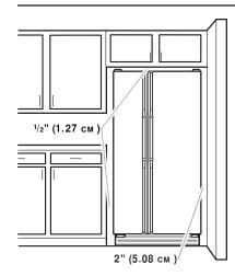
To ensure proper ventilation for your refrigerator, allow for ½" (1.27 cm) of space on each side and at the top. Allow for 1" (2.54 cm) of space behind the refrigerator. If your refrigerator has an ice maker, allow extra space at the back for the water line connections. When installing your refrigerator next to a xed wall, leave a 2" (5.08 cm) minimum space on each side (depending on your model) to allow the doors to swing open.
