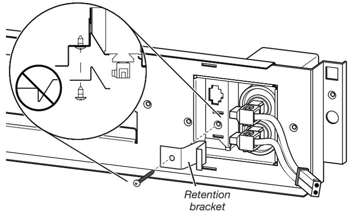
5. Secure the blower motor strain relief, near the quick connection end, to the blower electrical terminal cover with the two provided screws.
