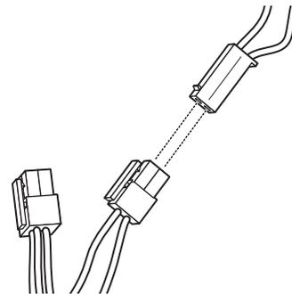
7. Locate the 4-pin connector on the blower motor wire and plug it into the terminal connection point directly behind the capacitor storage tray.
