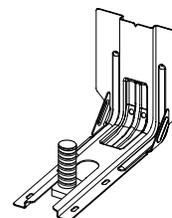
6. Visually check that there is an air gap between the Blower Motor Cover and the bottom of the range to ensure proper blower motor ventilation.
