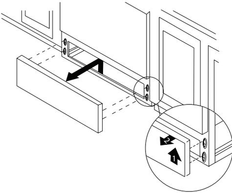
2. Unlatch and remove the Enclosure Front.
