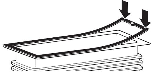
6. Apply blower motor cover to the blower. Slightly spread the cover retainer spring to allow the cover to drop into position on the blower motor. Ensure the blower cover retainer ring is securely locked in place.
