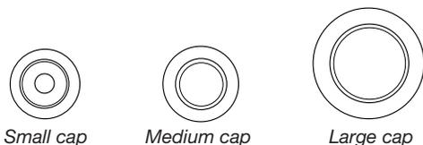
Burner caps should be level when properly positioned. If burner caps are not properly positioned, surface burners will not light. The burner cap should not rock or wobble when properly aligned.
