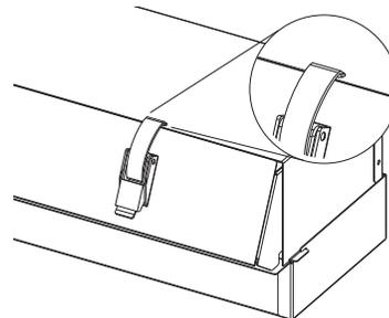
8. Replace the Front Lower Access Panel by aligning the studs with the keyhole slots on the range. Press the access panel forward into the slots and push downward to engage the studs.
