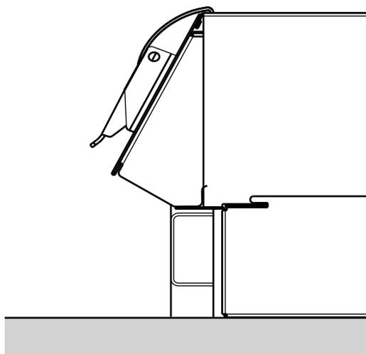
**NOTE:** If the Lower Filter Enclosure is below the Lower Front Frame Cross Support, the blower may need to be shimmed.
