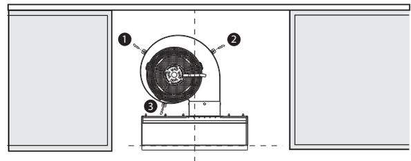
**NOTE:** If the range height adjustment is significant, the blower may need to be shimmed to ensure proper installation.
