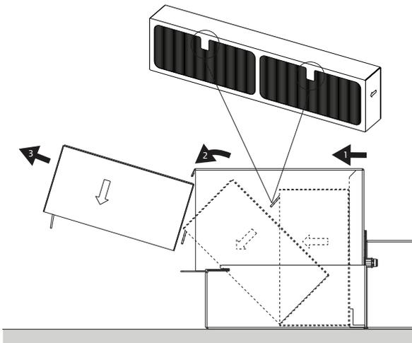
4. Thoroughly clean and dry the filter housing. You can clean the housing with a paper towel and household cleaners or with a cloth and warm soapy water. No special cleaners are required.
