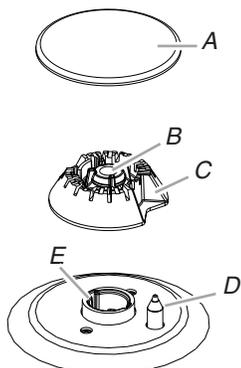
A. Burner cap      D. Igniter electrode
