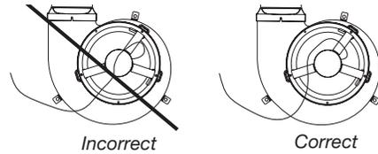
7. Rotate blower motor cover so the bellows are facing towards the right of the installation, and position the bellows so the bellow flange is facing the floor as illustrated.
