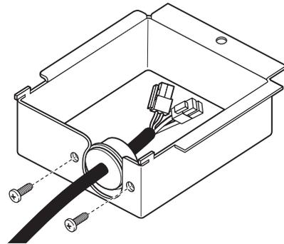
6. Locate the two-pin connector on the blower motor wire harness and connect it to the two-pin capacitor connector.
