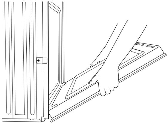
5. Using two hands, grasp the edges of the oven door. Lift and pull the oven door toward you and remove. You may need to gently shift door from side to side as you pull.
