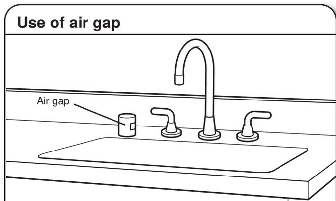
If required, the air gap should be installed in accordance with the air gap installation instructions. When you are connecting the air gap, a rubber hose (not provided) will be needed to connect to the waste tee or disposer inlet.
