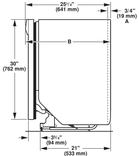
A. Insulation may be compressed (not used on all models).
