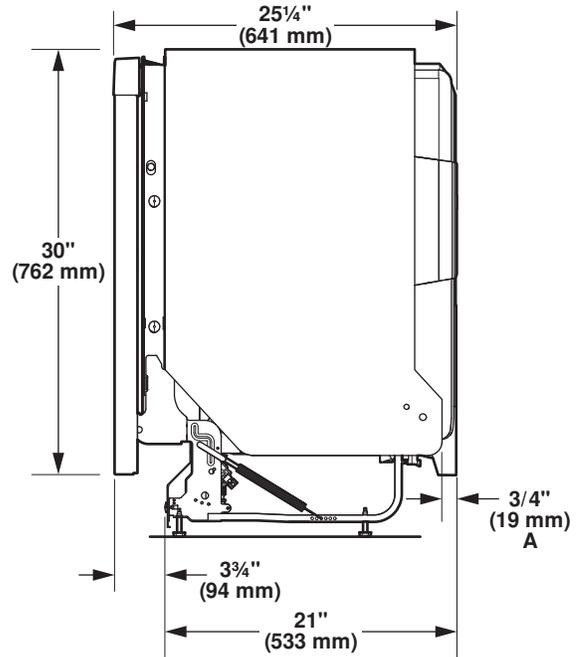
A. Insulation may be compressed (not used on all models).
