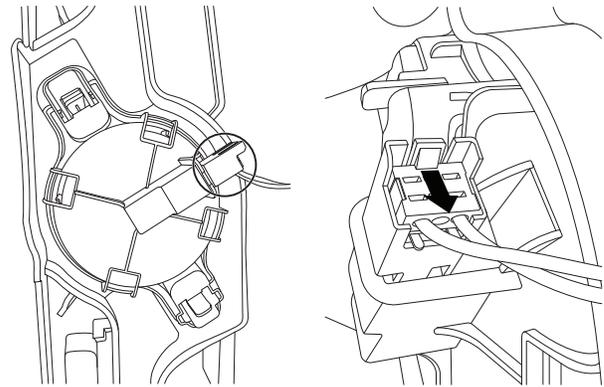
Check that the power supply wire or cord does not touch dishwasher motor or the lower part of the dishwasher tub.
