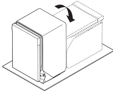
**Helpful Tip:** Remove all internal shipping material, drain hose, installation kit, and handle (if included,) before laying on it's back, and do not remove film on the door at this time.
