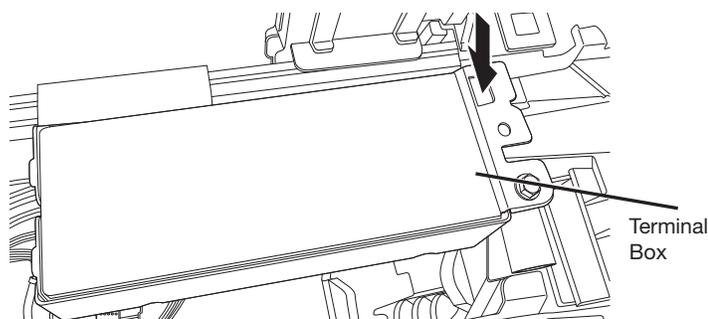
To remove the terminal box, depress the plastic latch, slide the box toward the left of the unit along the metal tube and rotate the left side of the box forward. Make sure that the product wiring is still attached within the terminal box
