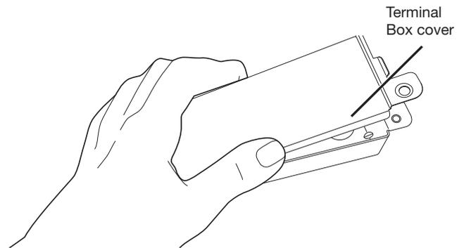
Using 1/4" (6.4 mm) nut driver remove the screw holding the terminal box cover. Remove the cover by lifting it out of the box. Keep the cover for later use.
