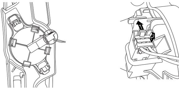
To remove the float switch wire, gently push the connector latch (1) and then pull the connector (2) out of the housing. The float itself should not be removed from the tray.
