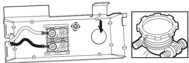
Install a UL Listed/CSA Approved metallic strain relief. Make sure screw heads are facing up when tightening conduit nut. Strain relief is provided with the power cord kit.
