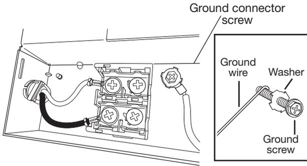
Route power cord through strain relief in the back of the terminal box. Remove the ground connector screw on the raised floor inside the box and place it through the ring terminal of the green ground wire of power cord. If wire has no ring terminal, bend a loop in the end of the wire. Reattach and tighten the ground connector screw to the raised floor of the box.
