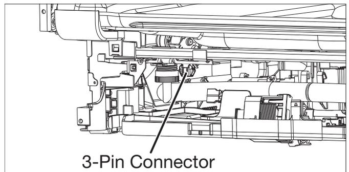
On some models, a service connection wire with a 3-pin connector is intentionally left unplugged and tucked behind the access panel. This is provided for use by the service technician.
