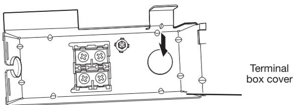
Tighten strain relief screws to secure cord.
