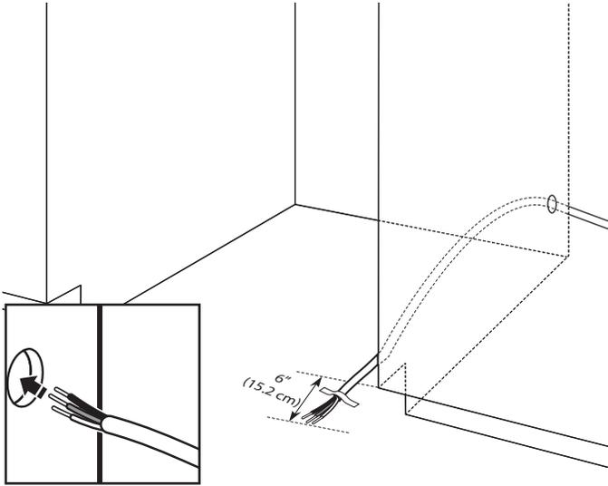
If installing with direct wire, route the cable as shown. Do not connect the wire to the product at this time. This connection will be made later, after the unit is installed into the cabinet opening.
