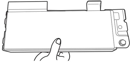
Place wires inside terminal box. Replace the cover by inserting the hooks of the terminal cover into the slots in the floor of the terminal box and sliding the cover tight against the back wall where wires come in. Make sure wires are tucked inside the box and not pinched by the cover. Put the terminal box back on the crossbar and push to the right so terminal box snaps into the plastic side member.
