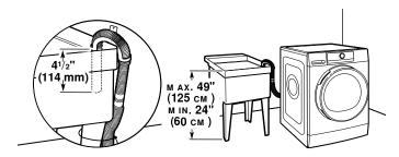
Minimum capacity: 20 gal. (76 L). Top of laundry tub must be at least 24" (60 cm) above oor; install no higher than 49" (125 cm) from bottom of washer.
