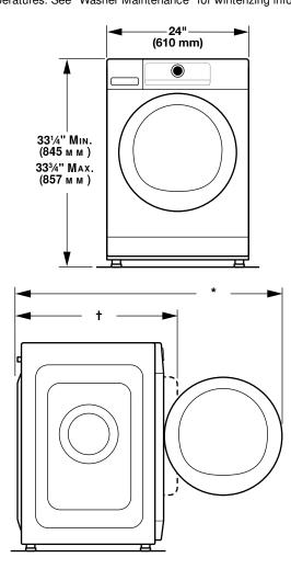
\*2.3 cu. ft. models: 42<sup>15</sup>/16" (1091 mm) 1.9 cu. ft. models: 41<sup>5</sup>/8" (1057 mm)
