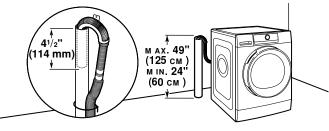
Minimum diameter for a standpipe drain: 2" (51 mm). Minimum carryaway capacity: 17 gal. (64 L) per minute. A 1/4" (6 mm) diameter to 1" (25 mm) diameter Standpipe Adapter Kit is available (Part Number 3363920). Top of standpipe must be at least 24" (60 cm) high; install no higher than 49" (125 cm) from bottom of washer. If you have an overhead sewer and need to pump higher than 96 inches, a sump pump and associated hardware are needed. See "Alternate Parts."
