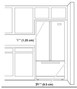
To ensure proper ventilation for your refrigerator, allow for a 1/2" (1.25 cm) of space on each side and at the top. Allow for a 1" (2.54 cm) space behind the refrigerator. If your refrigerator has an ice maker, allow extra space at the back for the water line connections. When installing your refrigerator next to a xed wall, leave a  $3^{3}/_{4}$ " (9.5 cm) minimum space between the refrigerator and wall to allow the door to swing open.
