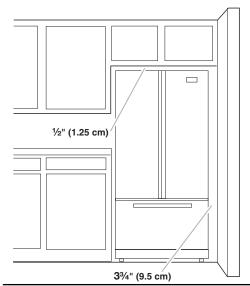
To ensure proper ventilation for your refrigerator, allow for a 1/2" (1.25 cm) of space on each side and at the top. Allow for a 1" (2.54 cm) space behind the refrigerator. If your refrigerator has an ice maker, allow extra space at the back for the water line connections. When installing your refrigerator next to a fixed wall, leave a  $3^3/4$ " (9.5 cm) minimum space between the refrigerator and wall to allow the door to swing open.
