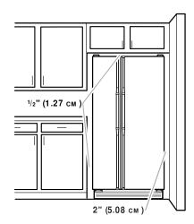
IMPORTANT: This refrigerator is designed for indoor household use only. To ensure proper ventilation for your refrigerator, allow for a ½" (1.27 cm) space on each side and at the top. Allow for 1" (2.54 cm) of space behind the refrigerator. If your refrigerator has an ice maker, make sure you leave some extra space at the
