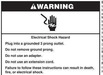
**Electrical:** A 115 V, 60 Hz, AC only, 15 A or 20 A fused, grounded electrical supply is required. It is recommended that a separate circuit serving only your refrigerator be provided. Use an outlet that cannot be turned off by a switch. Do not use an extension cord.
