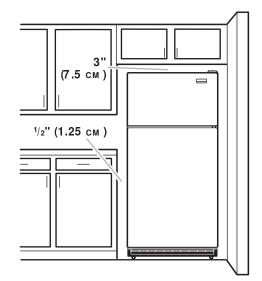
To ensure proper ventilation for your refrigerator, allow for a  $\frac{1}{2}$ " (1.25 cm) space on each side. Allow 3" (7.5 cm) of space between overhead cabinets and refrigerator top. Allow at least 1" (2.5 cm) between back of cabinet and the wall. If your refrigerator has an ice maker, make sure you leave some extra space at the back for the water line connections.
