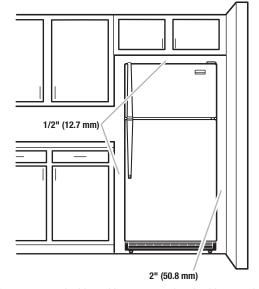
To ensure proper ventilation for your refrigerator, it is recommended to allow a 1/2" (1.27 cm) space on each side and between overhead cabinets and refrigerator top. Allow at least 1" (2.54 cm) between back of cabinet and the wall. If your refrigerator has an ice maker, make sure you leave extra space at the back for the water line connections.
