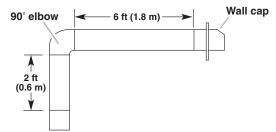
The following example falls within the maximum recommended vent length of 35 ft (10.7 m).
