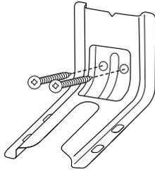
5. Using the Phillips screwdriver, mount anti-tip bracket to the wall or floor with the two #12 x 1<sup>5</sup>/<sub>8</sub>" screws provided.
