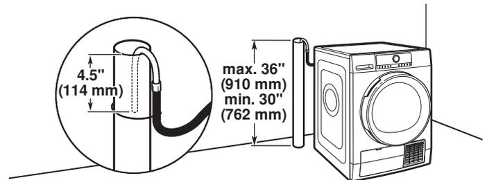
Minimum diameter for a standpipe drain: 2" (51 mm). Top of standpipe must be at least 30" (762 mm) high; install no higher than 36" (910 mm) from bottom of dryer.
